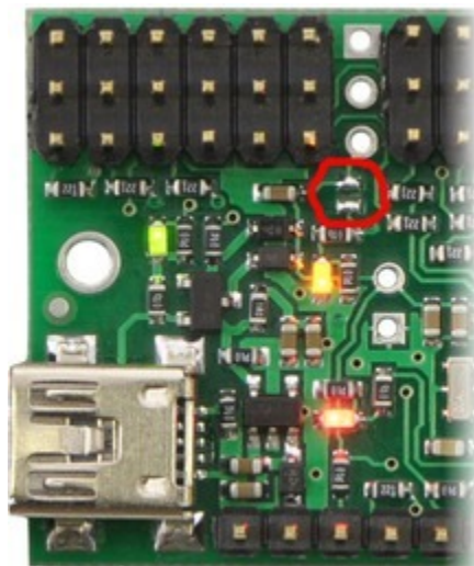
Bootloader pads for the Mini Maestro 12-, 18-, or 24-Channel USB Servo Controller.
